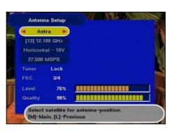
This menu is intended solely for service purposes and, if need be, i.e. if no measuring instrument is available, it can be used to align the antenna (satellite dish)
